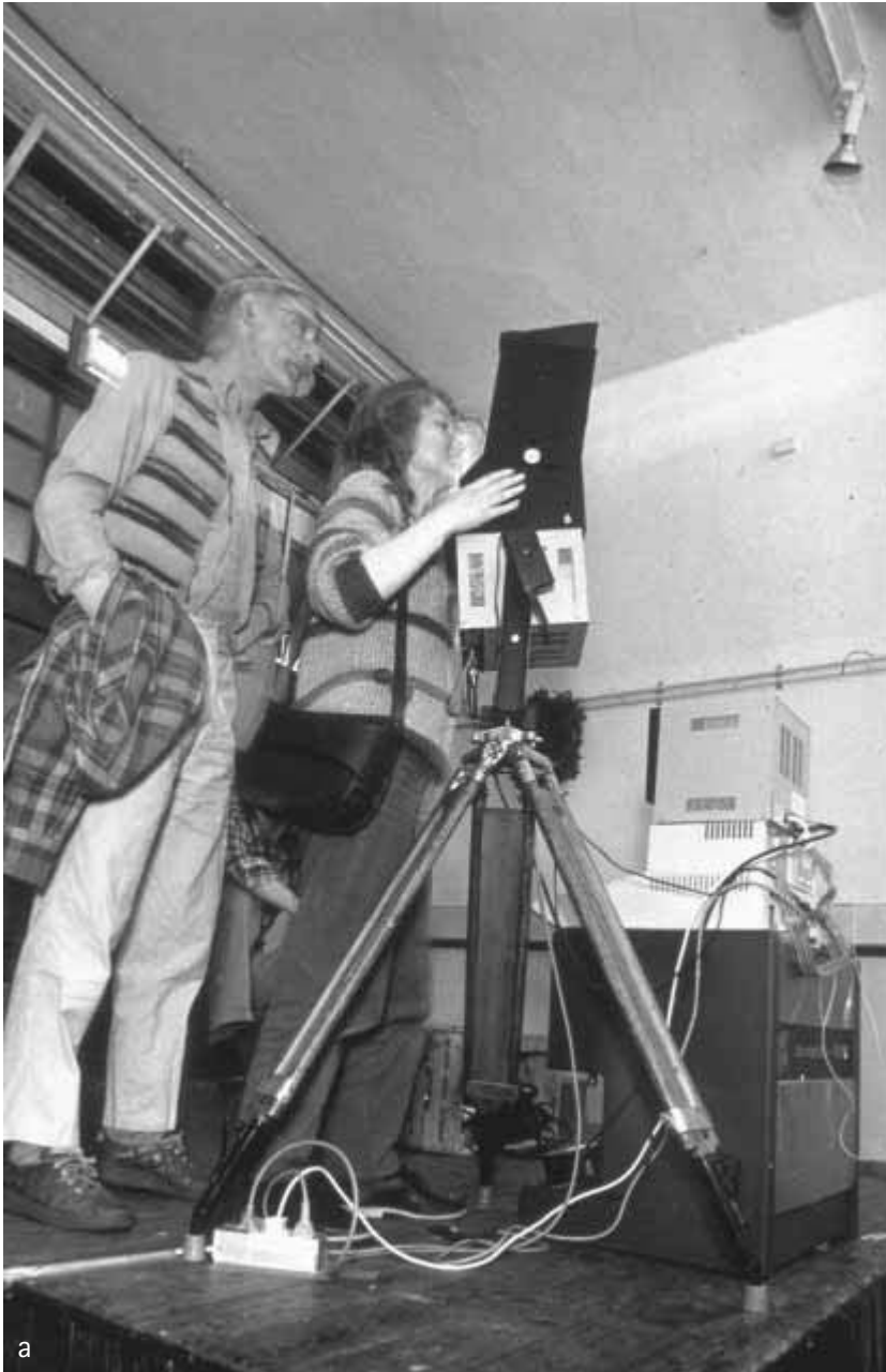
Figure 2.7 Jeffrey Shaw, Virtual Projection System (1983). Interface platform combining semi-transparent mirror and computer screen; permits viewer to rotate a cube projected within the image space. (a) Close-up of optical interface machinery. (b) Image of cube as seen through Virtual Projection System .
